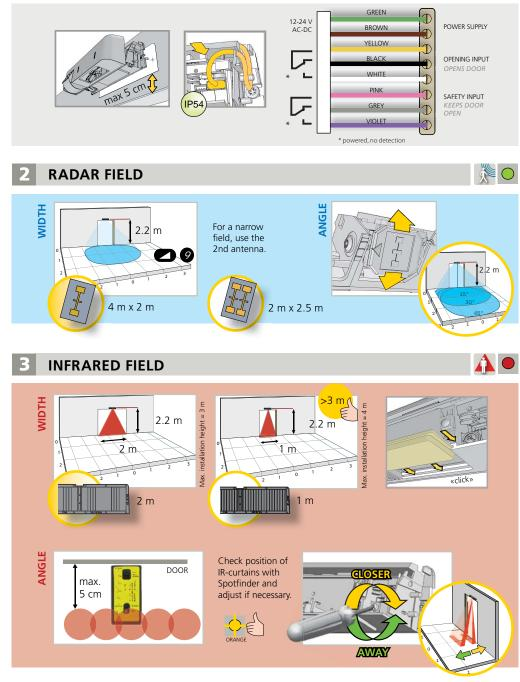
TIP: Launch an ASSISTED SETUP to verify wiring, position of the curtains and correct functioning of the sensor.
