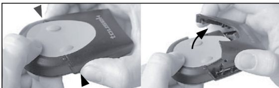
Fig. 3 Take the cover of the transmitter between thumb and forefinger and press the cover together and upwards.
